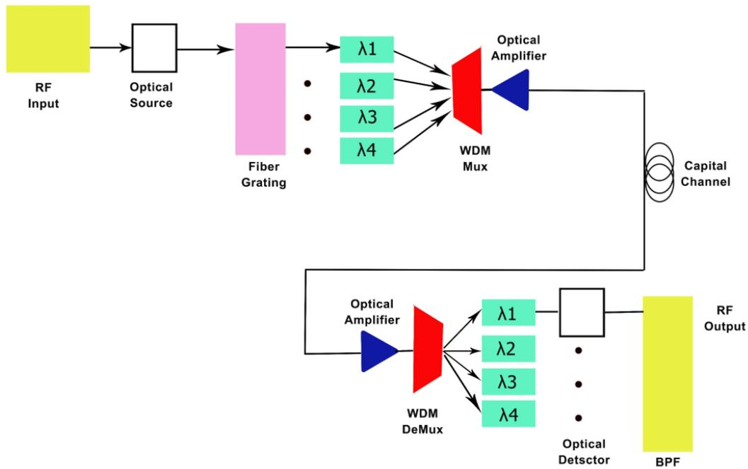
**Figure 2.11** Diagram of WDM RoF System[35]
