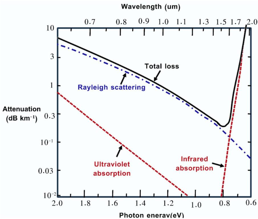
**Figure 2.4** The absorption of material losses in silica glass fibers [21]
