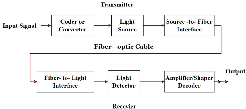
**Figure 2.2** Basic fiber optical communication system [24]
