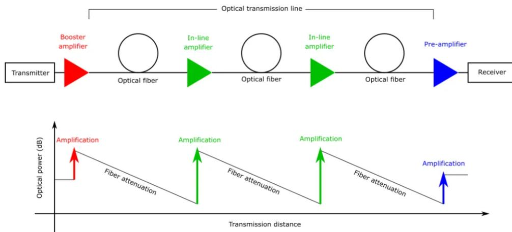
**Figure 4.7** EDFA Utilization In Optical Fiber Communication [57]
