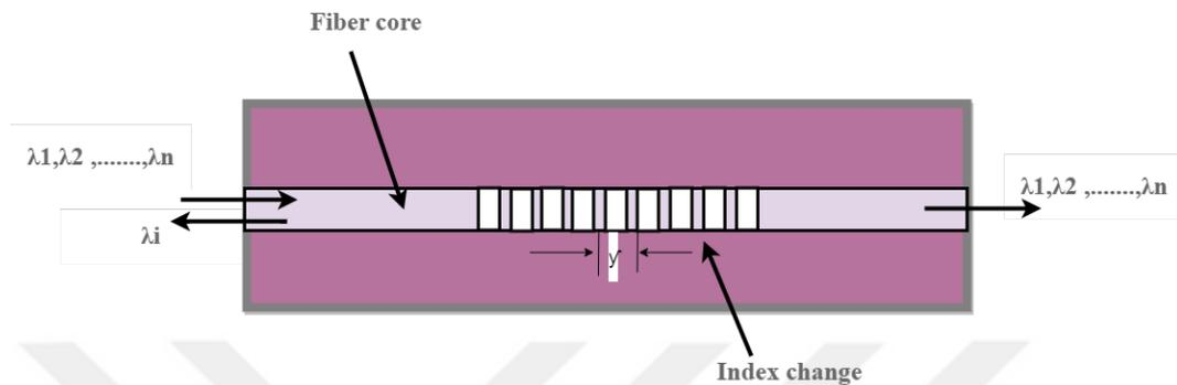
**Figure 3.4** Schematic View of FBG[45]
