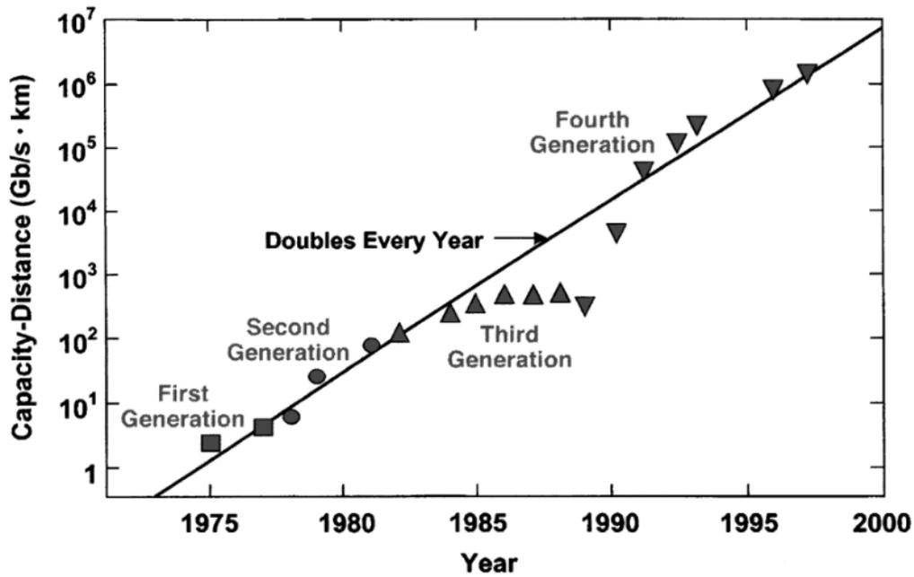
Figure 2.1 The generation of development of optical communication system [22]
