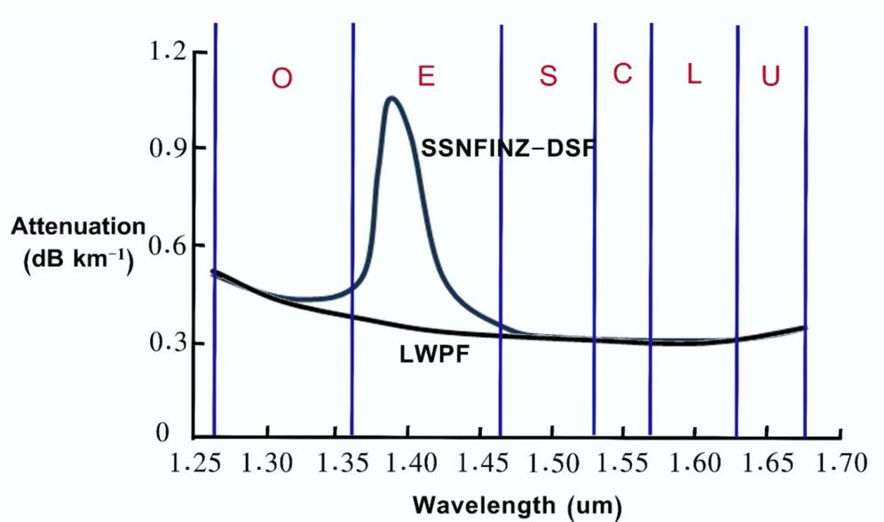
**Figure 2.3** The absorption of material losses in silica glass fibers [22]
