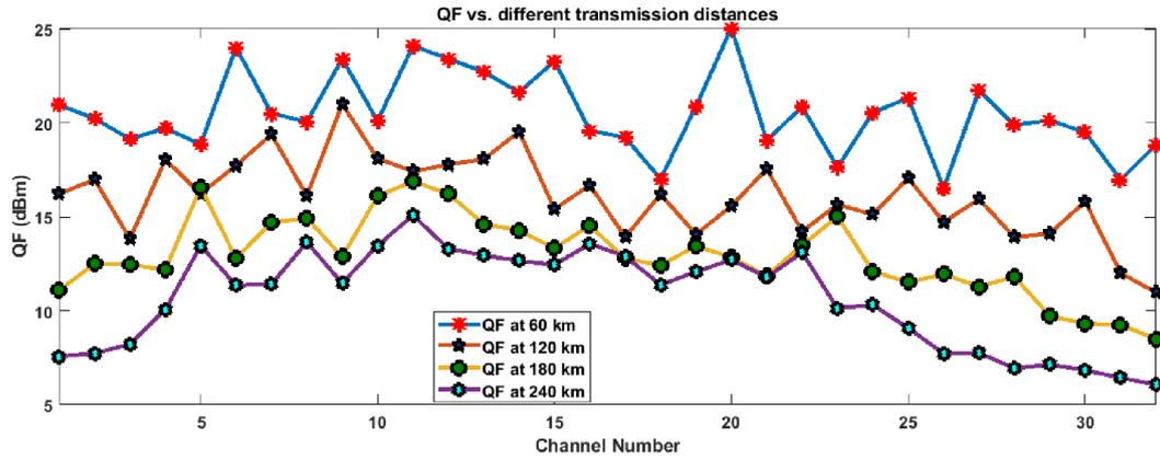
**Figure 5.1** The Relation of QF vs. Different Transmission Distances.
