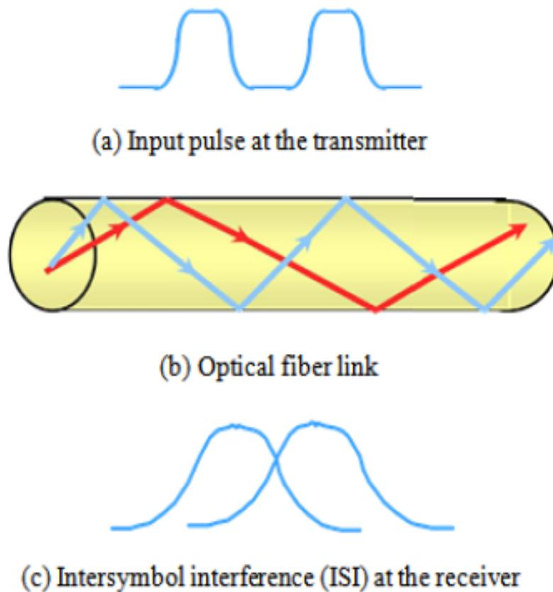
**Figure 3.2** ISI Effect On The Transmitted Pulses [40].
