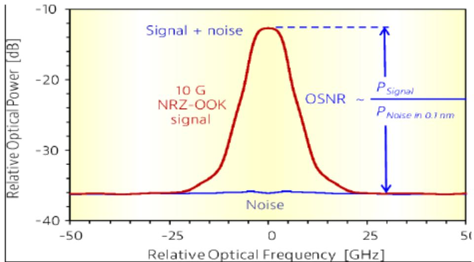
**Figure 2.7** Typical example of calculation of the OSNR [26]
