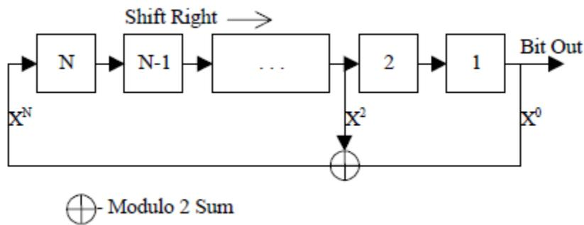
**Figure 4.3** Example of The Internal Circuit For a Type of PRBS[53]
