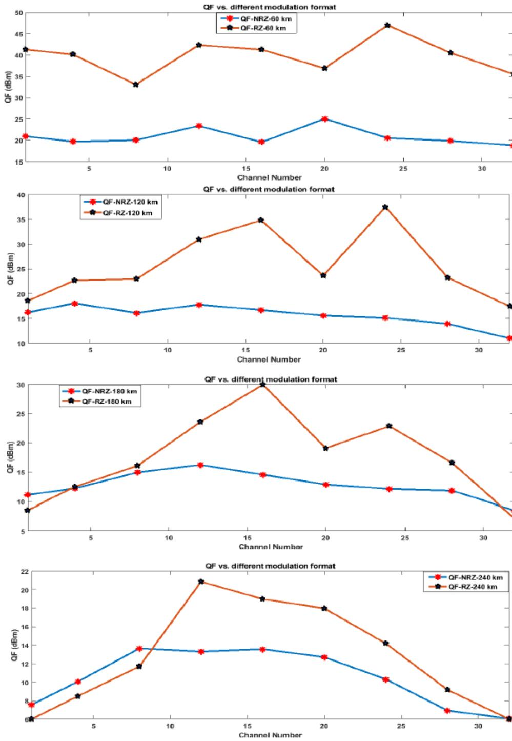
**Figure 5.5** QF vs. Different Modulation Format (a) 60 km, (b) 120 km, (c) 180 km and (d) 240 km.
