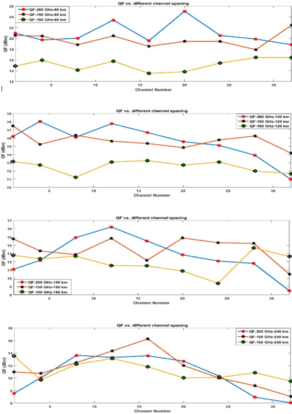
Figure 5.3 QF Vs. Different Channel Spacing For (a) 60 km, (b) 120 km, (c) 180 km and (d) 240 km.
