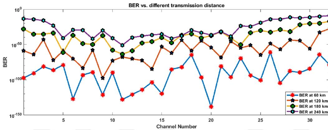
**Figure 5.2** The Relation of BER vs. Different Transmission Distances.
