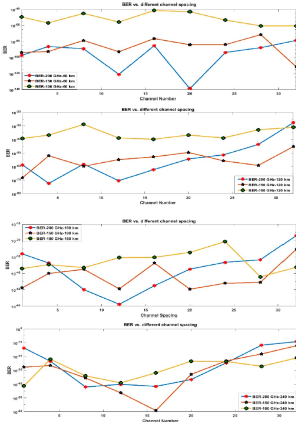
**Figure 5.4** BER vs. Different Channel Spacing For (a) 60 km, (b) 120 km, (c) 180 km and (d) 240 km.
