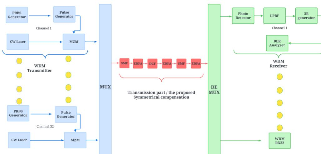
**Figure 4.9** The Schematic View of The Proposed System
