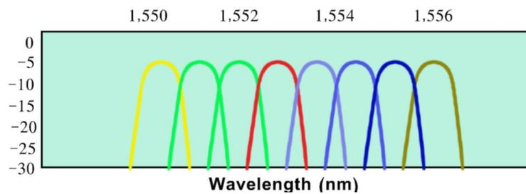
**Figure 2.12** Comparison in Channel Spacing Between CWDM and DWDM [37]
