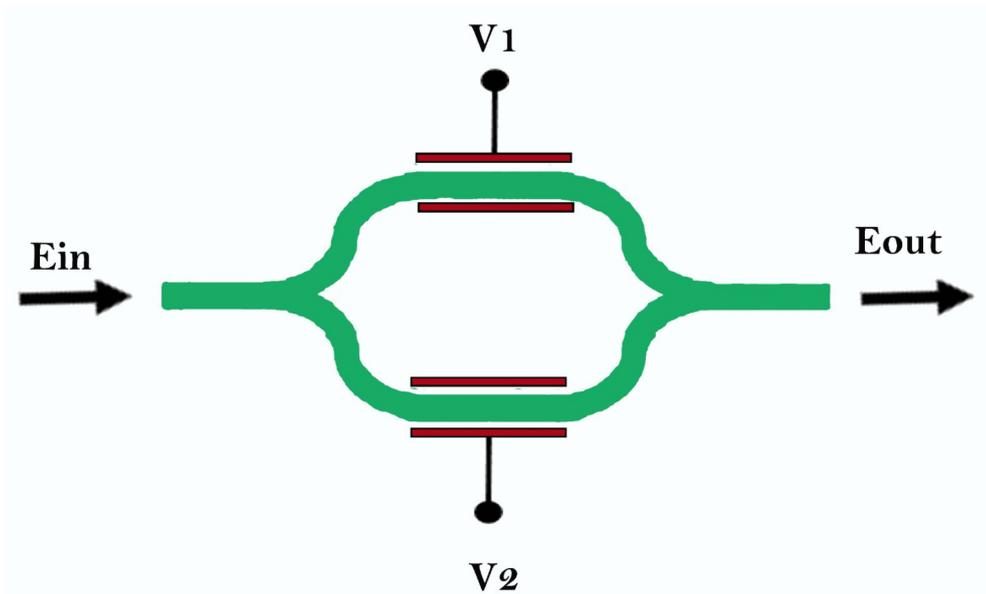
**Figure 4.5** The Structure of The MZM [55]
