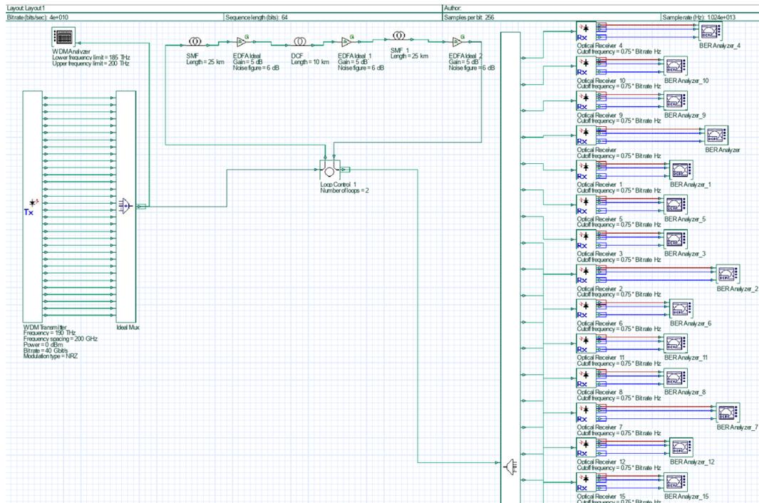
**Figure 4.8** The Proposed System Designed Using Optisystem.
