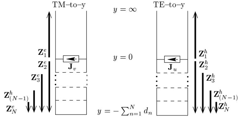
Figure 2: Equivalent transmission lines for the TM and TE fields
