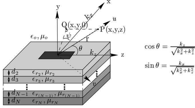
Figure 1: Cross-section of a multilayered microstrip resonator
