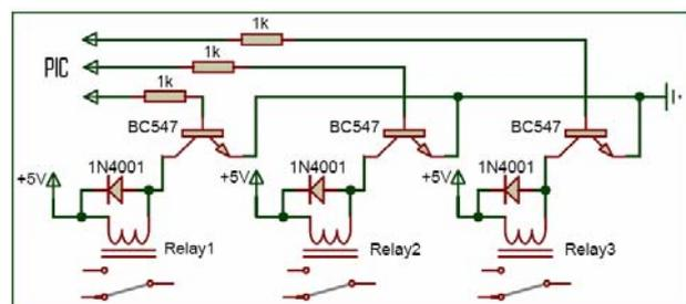
Fig 8 Relay driver circuit
