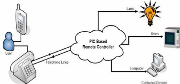
Fig. 1 Block diagram of remote controller system.
