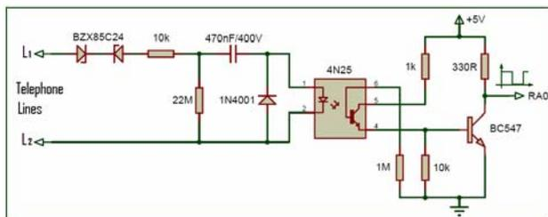
Fig. 5 Optical isolation circuit.
