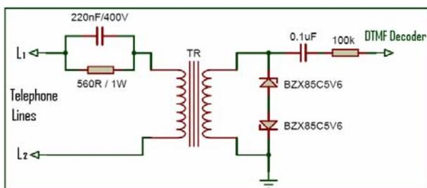
Fig. 6 Magnetic isolation circuit.
