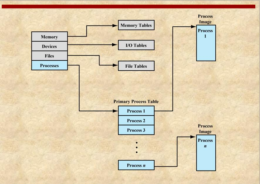
Figure 3.11 General Structure of Operating System Control Tables
