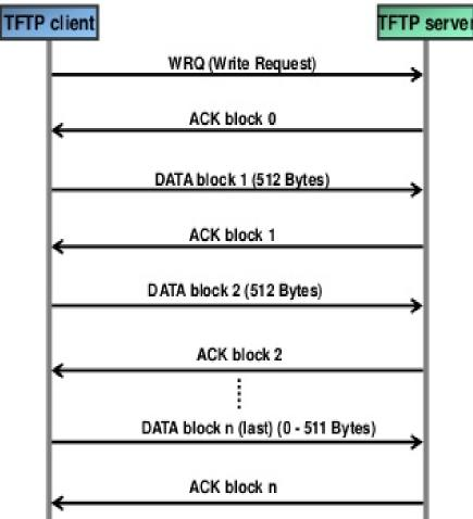
The transfer is initiated by a write request packet (WRQ).
