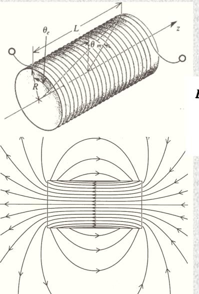
The selenoid is close-wound of lenght *L* with *N'* turns per meter, and its Radius is *R*. At the center
