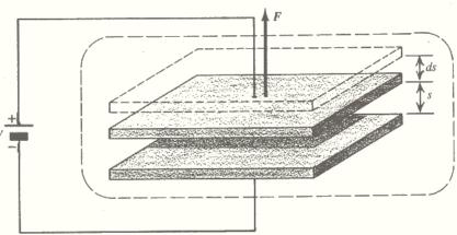
Assume that the distance s increases by ds, and apply the principles of the virtual work The increase in the electric energy of the capacitor is
