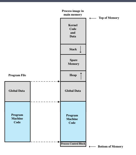
Figure 10.4 Program Loading into Process Memory
