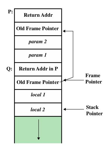
**Figure 10.3 Example Stack Frame with Functions P and Q**
